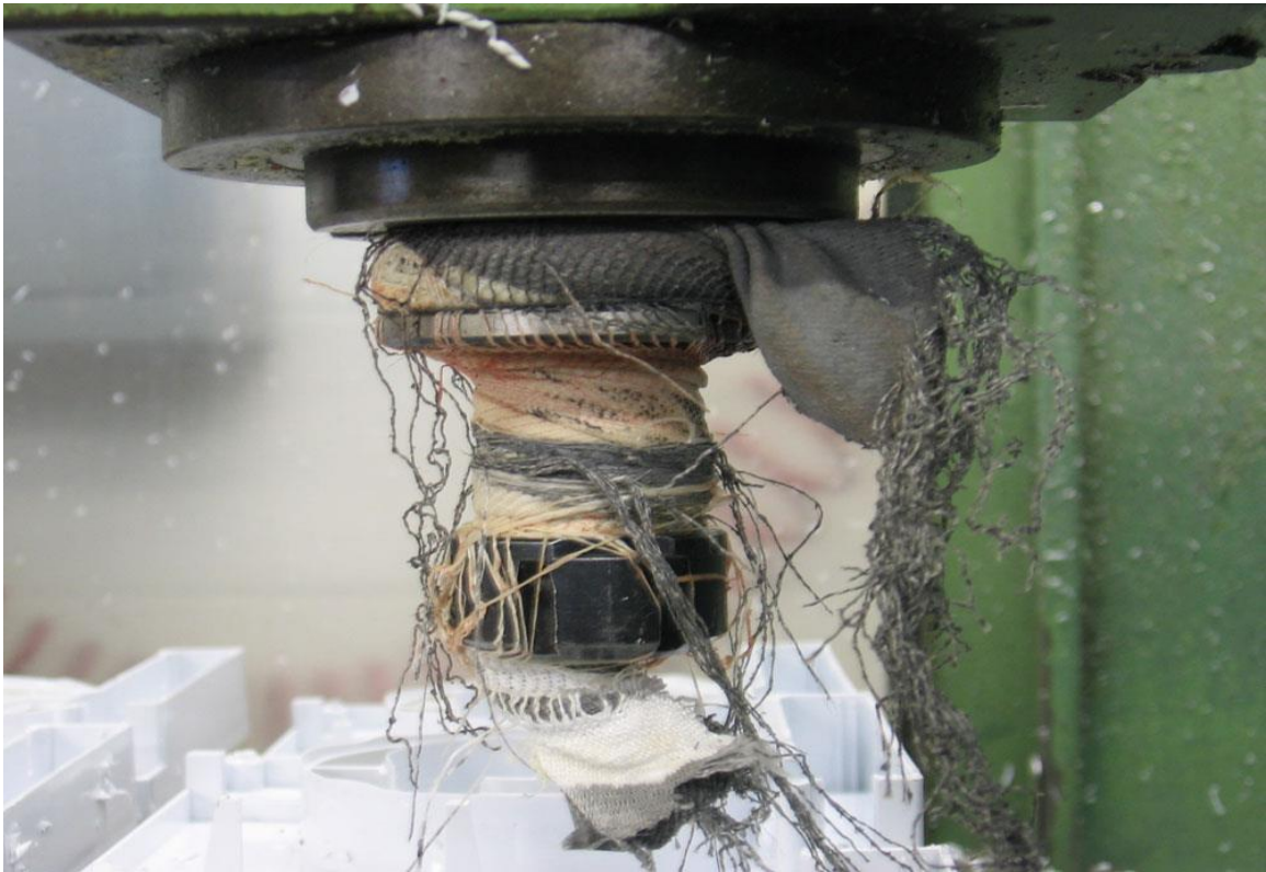
Figure 3.3.2.2: Example of clothing caught in machinery.
